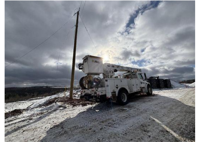
Line truck set to install the overhead line.
